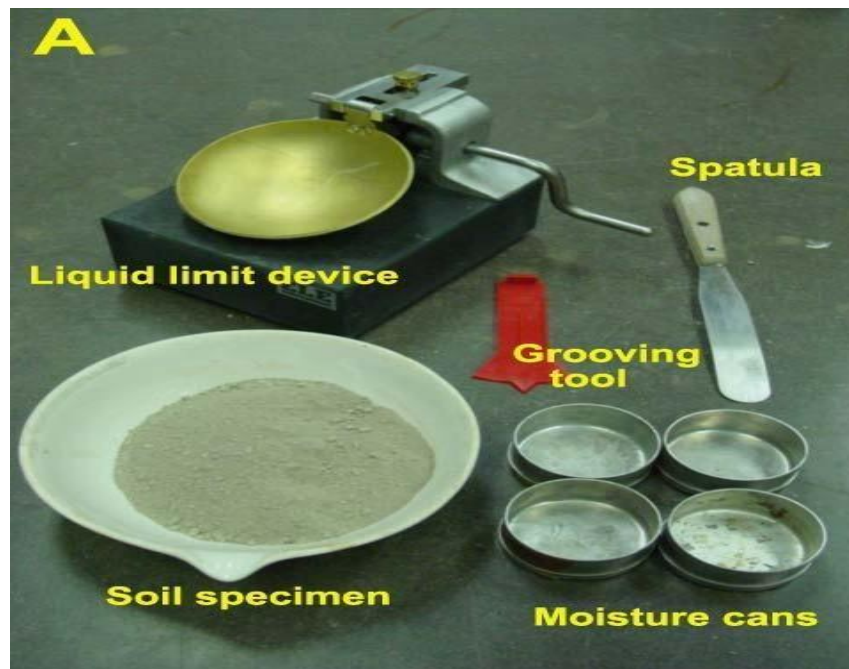
Fig: Shows Liquid limit test apparatus
