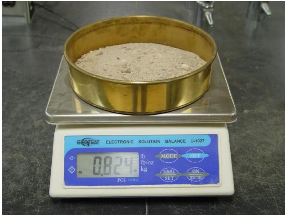
Fig: Illustrates Sieve Analysis test procedure
